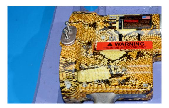
**Step 1:** Position the copper coated "Button" onto the housing of the unit as shown below. Start two RG-0046 Torx screws into the holes in the button.
