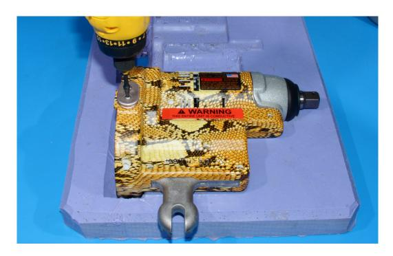
**Step 2:** Using the small drill motor with a T-15 drive bit, tighten the two screws into the housing to secure the button in place.
