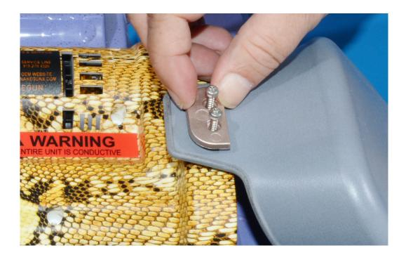
**Step 5:** Turn the Rattlegun assembly over so that the "Button" is facing downward. Position the battery boot and cap over the two screw holes in the housing as shown below.
