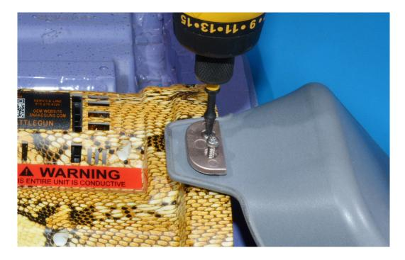
**Step 6:** Using the small drill motor with a T-15 drive bit, tighten the two screws into the housing to secure the Cap and Battery Boot in place.
